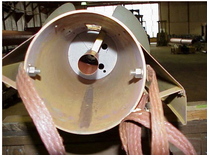
Figure 4: Pressure Protected Antenna After 30 Years of Service in Chicago
