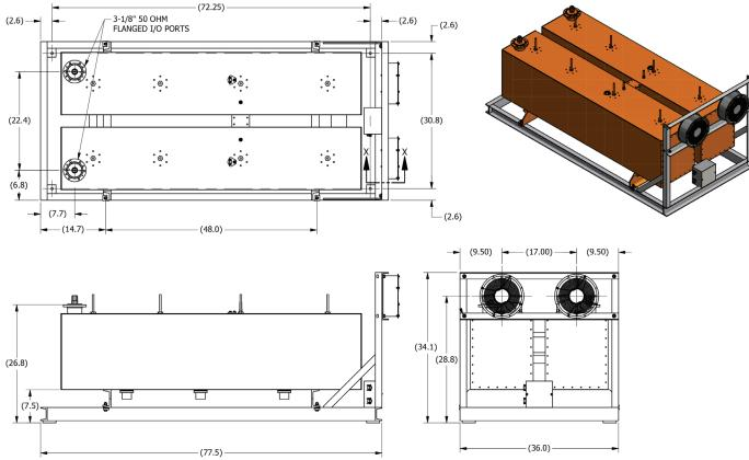
VF-H12500-83 Eight Section High Band VHF Band Pass Filter. Dimension shown in inches.
