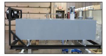
The VF-H12500-83 is a compact, eight section, high band VHF band pass filter that is adjustable for operating frequency, bandwidth, and mask slope. The filter can be configured to meet the requirements any standard digital or analog mask. This is a temperature compensated filter it maintains emissions compliance and an excellent input match from "cold start" and with variations in ambient temperature.
