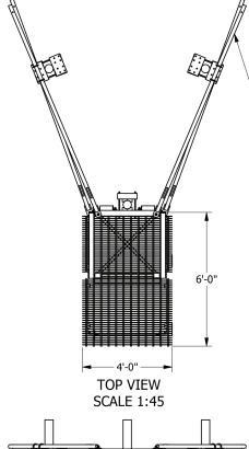
Weight 1/2-inch (13mm) Ice No Ice 625-lbm 283.5-kg 1100-lbm 499.0-kg **Effective Projected Area** Normal 1/2-inch (13mm) Ice No Ice 12.6-ft<sup>2</sup> 1.17-m<sup>2</sup> 15.4-ft<sup>2</sup> 1.43-m<sup>2</sup> **Transverse** 1/2-inch (13mm) Ice No Ice 20.4-ft<sup>2</sup> 1.90-m<sup>2</sup> 26.6-ft<sup>2</sup> 2.47-m<sup>2</sup>
