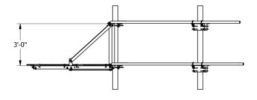
The ERI model ISA-04-06S is a galvanized steel leg mounted ice with standard models that includes tiebacks for uniform cross-section tower face sizes from 3.00-feet (914-mm), to 12.00-feet (3658-mm). Each ice shield includes leg mount brackets to attach to round tower members from 1.25-inch (32-mm) to 8.00-inch (203-mm) in diameter
