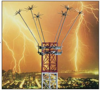
The Lightning Spur is a very efficient hybrid lightning dissipater. When operating as a shield it reduces the potential between the tower and storm cell by transferring electrical charge to the adjacent ionizing air molecules. This transference represents dissipation or the controlled leakage of the charge, thus reducing the probability of a lightning strike.
